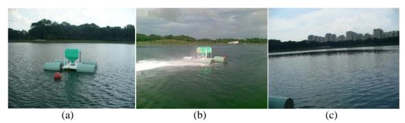
Figure 5. (a) Anchored Spreaders; (b) Automatic dosing of *WaterSavr* on the Reservoir; (c) *WaterSavr* (mono-layer) spreading
